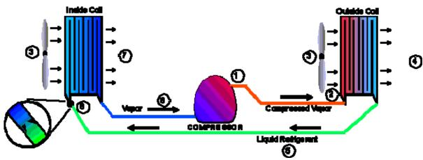
Air conditioning is really pretty simple when you get down to the basics. It is a sealed system composed of copper tubing, some electronics, and three basic components. A compressor and two heat exchangers or coils. The cycle goes like this;
